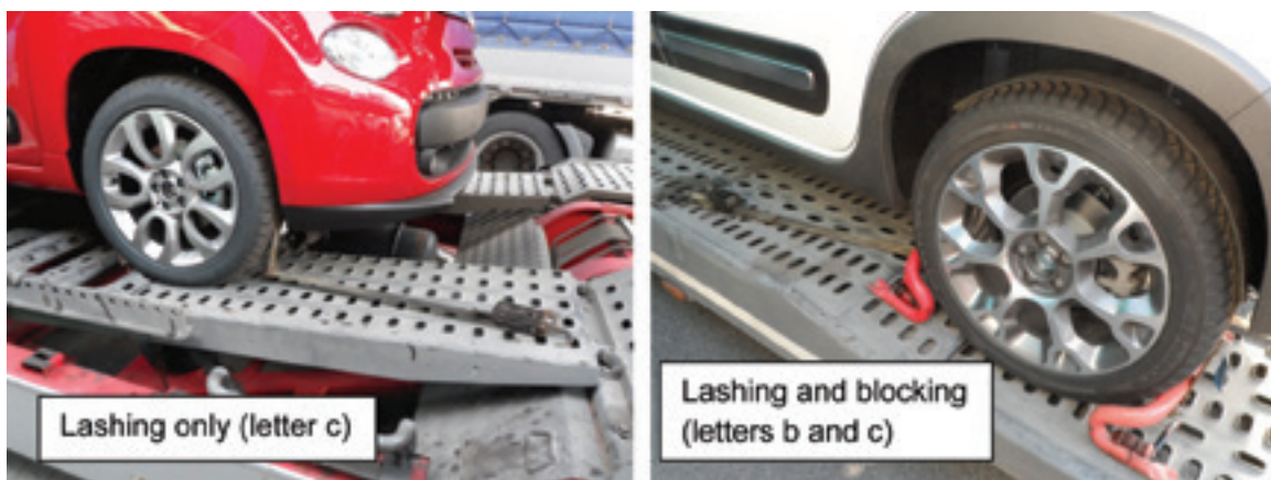
Figure 57: Securing arrangements for car transport
