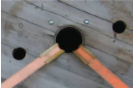
Figure 22: Protection at sharp edges
