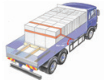
Figure 40: Spring lashing using a sling
