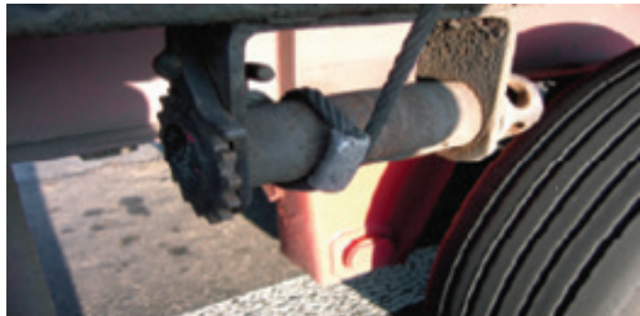
Figure 24: Steel wire rope tensioned by winch
