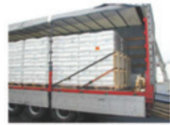
Figure 39: Spring lashing using pallets
