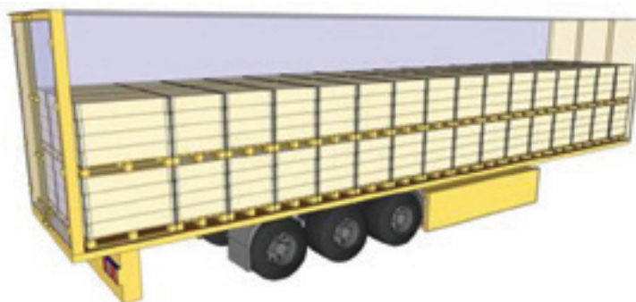
Figure 69: Stowing of pallets in XL coded vehicle
