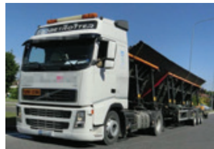
Figure 14: Steel plates transported under 45°
