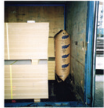
Figure 29: Air cushion for sideways blocking
