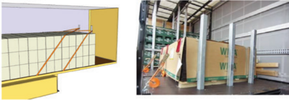
Figure 7: Stanchions used for blocking in forward direction
